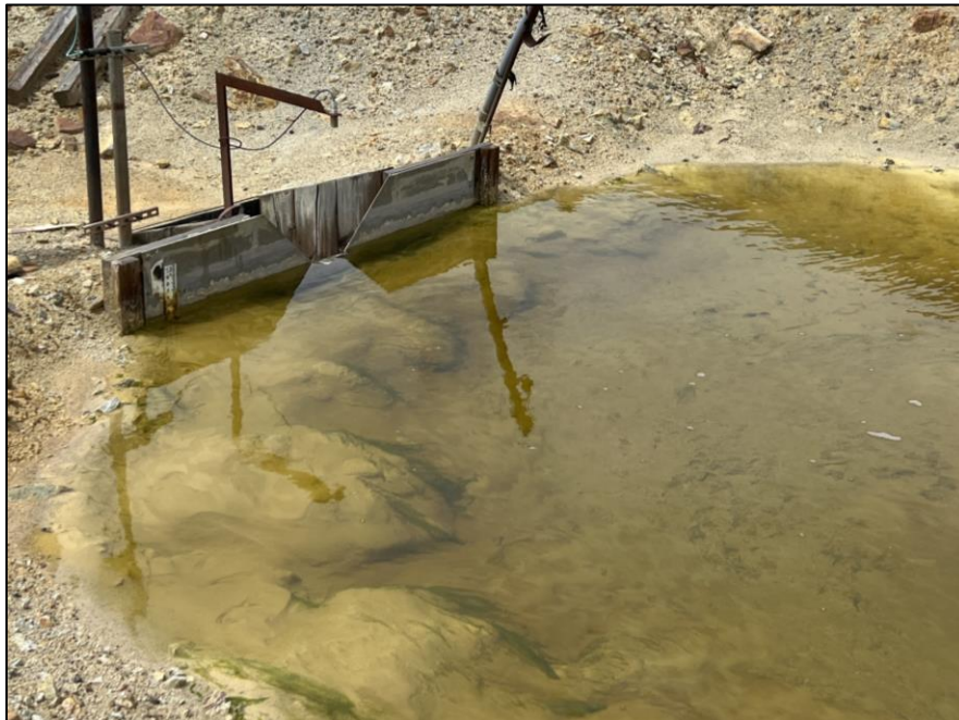
PHOTO 2 – June 12, 2023 – Seep 10 Weir and Staff Gauge reading slightly below 0.4.
