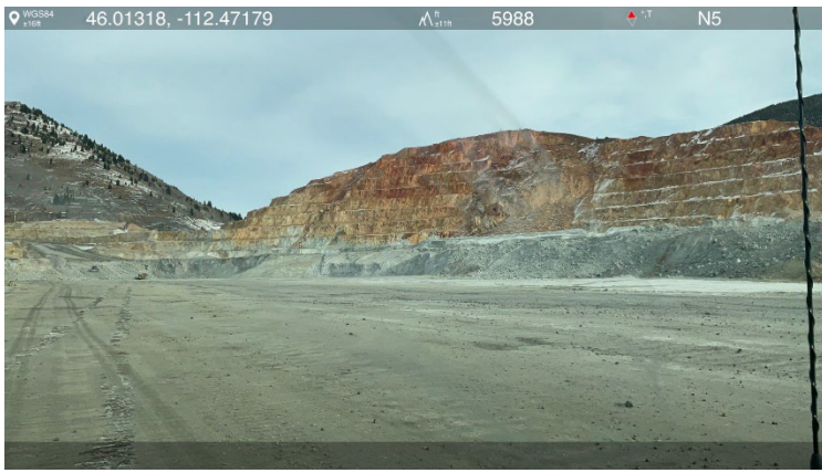
Photo 3- Note that the lateral extent of the failure was limited by a wide access road which separates the D East area from the deeper portions of the Continental Pit (to the left of this view). Photo 4- Vegetation removal and soil salvage are ongoing to the east of the highwall and this material is being stockpiled in other locations along the East Dump Complex, where it may be more easily accessed for future use during reclamation.
