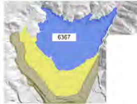
1 in 1,000 30-day Rainfall Event Total Pond Volume ~ 33,100 acre-ft Pond Elevation ~ EL. 6,367 ft
