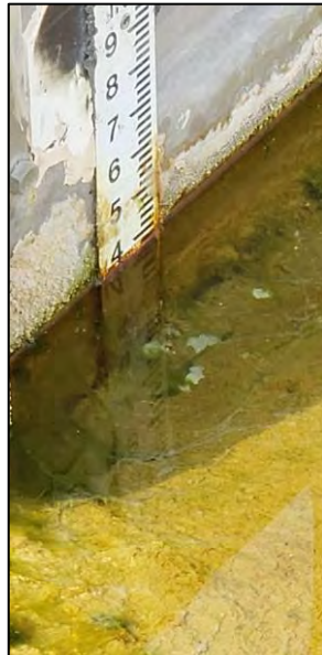
PHOTO 4 – Sep 16, 2020 – Seep 10 Staff Gauge reading slightly below 0.4.
