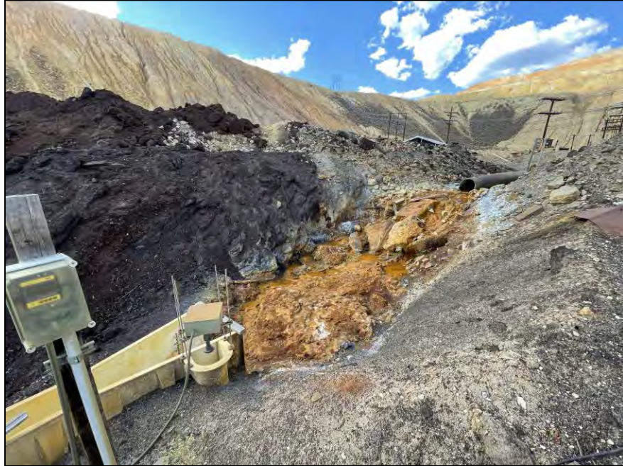
PHOTO 13 – Horseshoe Bend – Minor flows passing through the Precipitation Flume from the former Cell 10 Pump area
