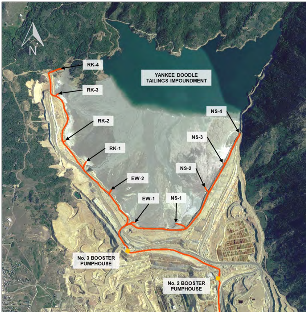
Figure 3.1 YDTI Tailings Discharge Locations
